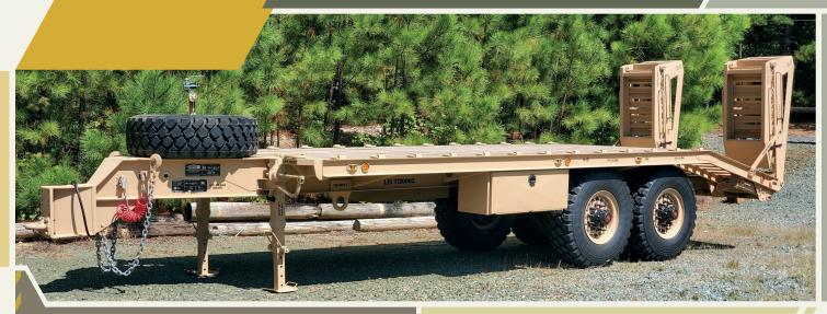
The M1269 Type II Light Engineer Utility Trailer (LEUT) is a heavy duty, off-road, pintle towed utility trailer providing equipment and ammunition transport capability.
